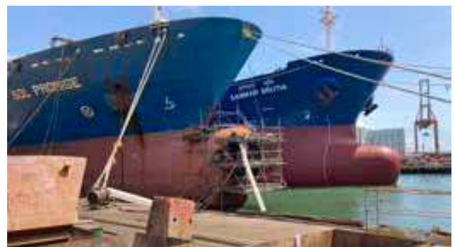
Figure 03: Bow damage repair on SOL Promise
