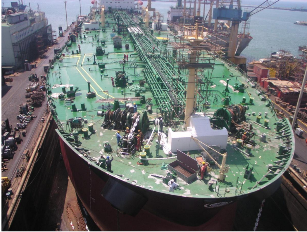
Vessel maneuvering in/out of the drydocks, with the aid of hauling winches.
