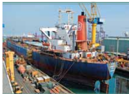
The MV. Sunrise in afloat condition during the dismantling process, the deck machinery and cranes removed.
