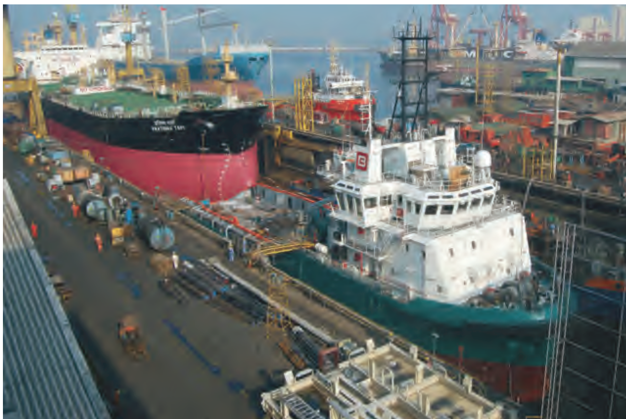
Multiple drydocking of vessels are the order of the day, Tanker Prathibha Tapi, OSV Bourbon Themis and a Dredger Costa Blanca accommodated simultaneously in 125,000 DWT capacity Drydock No. 04.
