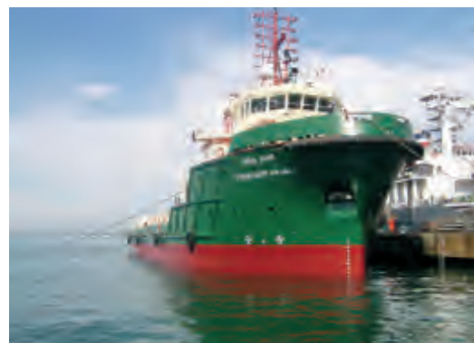
Greatship Anjali - 80 Ton Bollard Pull Anchor Handling Tug Supply Vessel built for Greatship India Limited.
